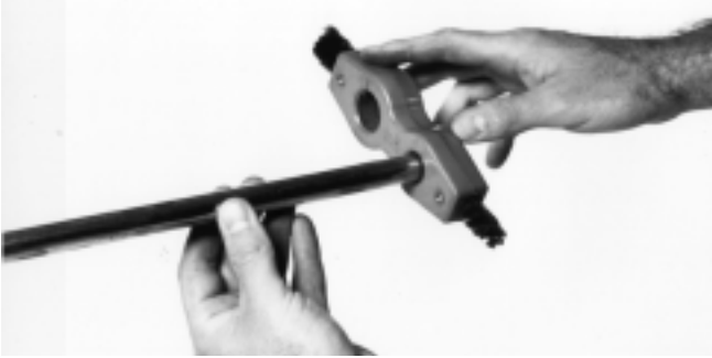
Figure 3 – Cleaning Copper Tube and Fittings
